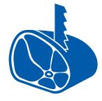
Always cut straight through the meat and never twist the Bandsaw Blade when operating. Do not push but let the Bandsaw Blade work itself through the meat with light pressure.
