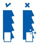
Never let the Bandsaw Blade scrapers come in contact with the saw teeth.
